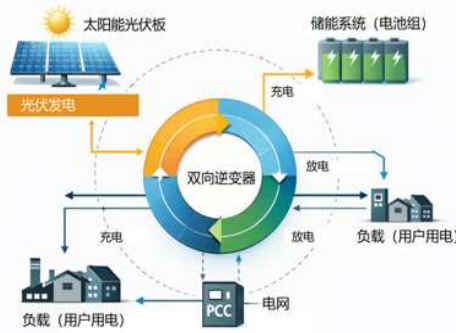
Fig. 2 Energy Flow and Operation Modes of PV-ESS System
